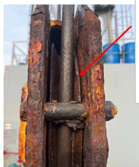
Hook block sheave, bearing, snap ring and collar (S00000348-007)
